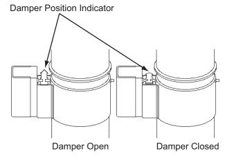
Fig. 11: Vent Damper Position Indicator
